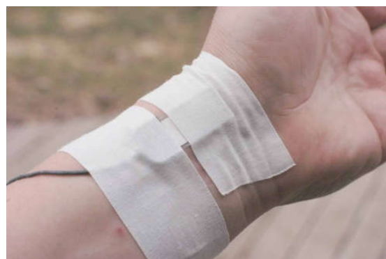
Fig. 3. Piezo film attached to the wrist with athletic tap
