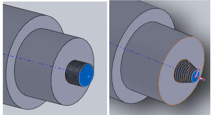
Figure 2. Tool used for the friction stir welding
