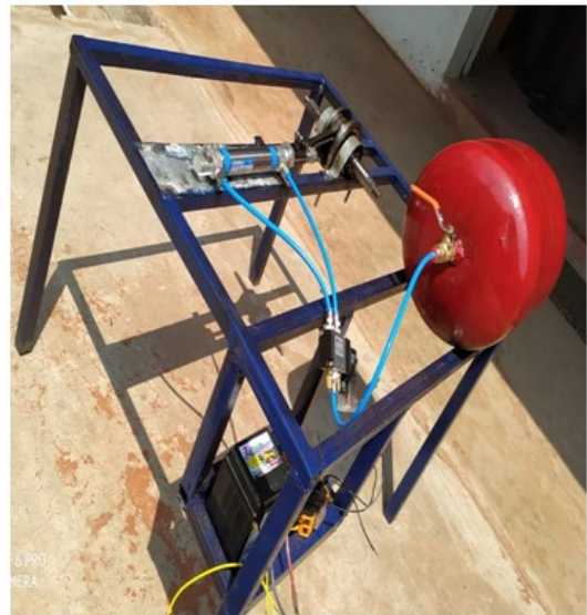
Fig. 9. Fabrication of Irrigation Pump Operated by Air Pressure
