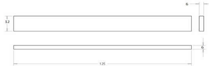
Figure 4. Flexural specimen according to ASTM standards prepared in CAD Software All Dimensions are in MM
