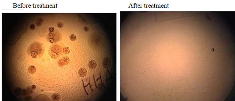
Figure 2. Example showing the disinfection of river water polluted by E coli using free radicals generated from zero valent iron powder reaction (25 ml of polluted water /0.2g of iron powder /air bubbling) River polluted (Hawaii –USA)
