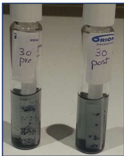
Figure 4. Pre-rinsing and post-rinsing samples formed colonies after incubation at 37°C for 48h
