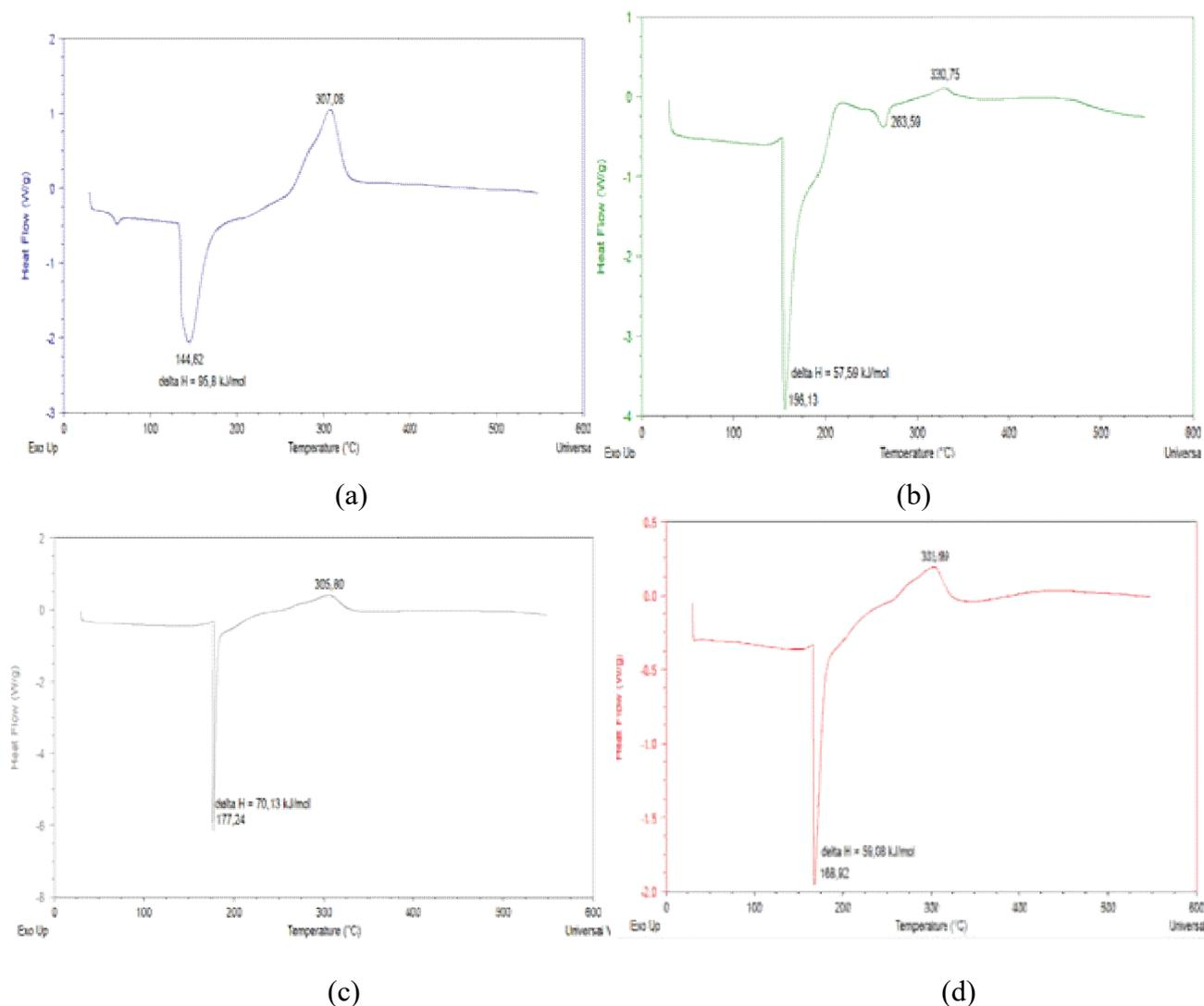
**Figure 1.** DSC thermograms of the materials: (a) gum arabic (b) anthocyanins, (c) particles obtained by spray-drying, and (d) particles obtained by lyophilization
