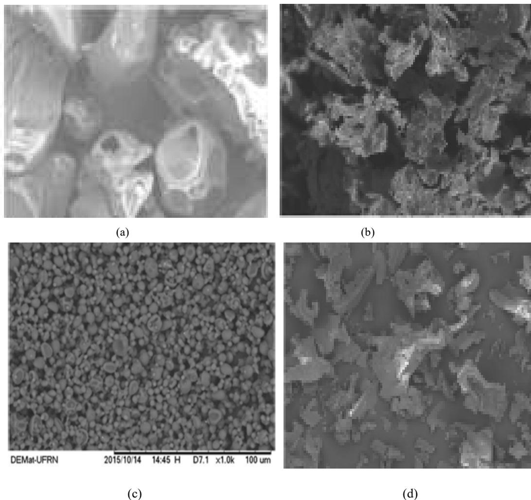
**Figure 2. Microphotographs of the materials: (a) gum arabic (b) anthocyanins, (c) particles obtained by spray-drying, and (d) particles obtained by lyophilization, at 1000 fold increase**
