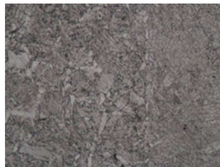
Fig.8 Microstructure of weld fusion zone
