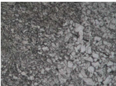
Fig.7 Segregation structure in Overheated zone
