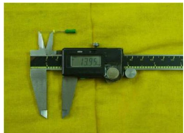
Figure 6b. Digital Vernier caliper measuring endodontic file
