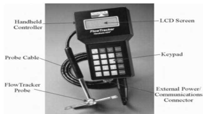
Fig.1. FlowTracker with 2D Probe
